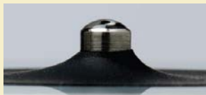
Droplet "attens out" on unconditioned pedestal
