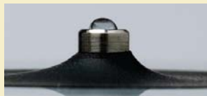
Droplet "beads up" on properly conditioned pedestal
