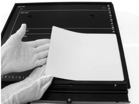
\* The phosphor stage is magnetic, so that it holds the storage phosphor screen in place.
